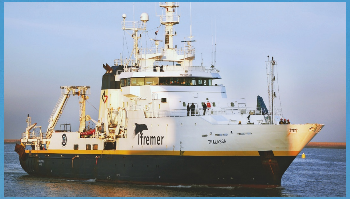
1996 "Thalassa" – This fisheries research vessel is used for missions such as population ecology and assessment of fished species. LowNoise thruster in the bow – conventional thruster in the stern.
